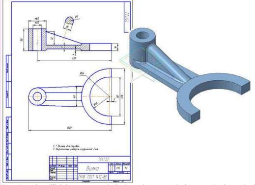
Based on the official purpose, technical requirements, design complexity and other factors, the method and material for obtaining the workpiece is selected. The material for obtaining the workpiece of this part can be either from cast iron of a number of grades, or several grades of steel.
