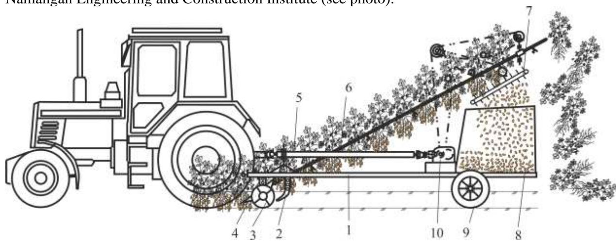
1-rama; 2 knives; 3 front base wheels; Router 4; 5-cardant extension; 6-pin clamp tape extension; 7 comb-suckers; 8-bunker;
